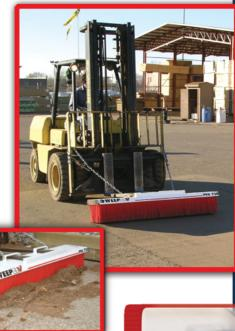
FORKLIFT: Easily hooks to cutting edge of any bucket or fits over fork times. Positive lockdown with forged chains and binders.
